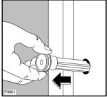
Remove the polystyrene block from the bottom of the machine and release the two plastic bags.
